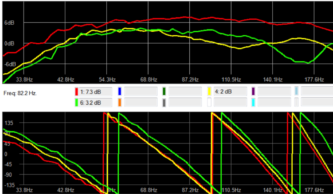
Figure 14: Red: Mono cluster, Yellow: Inverse stacked cardioid, Green: 2 in line cardioid
