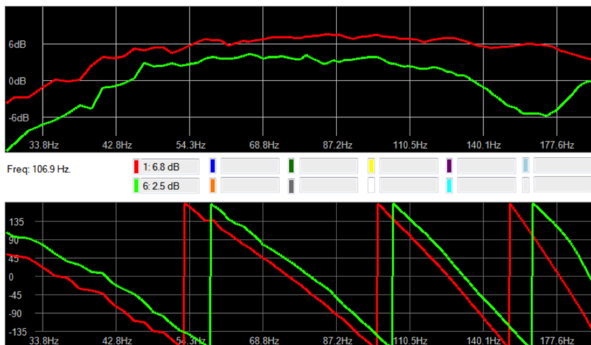
Figure 10: Red trace: mono cluster. Green trace: 2 in line cardioid. Measurement taken at 12m (36 ft) of distance.
